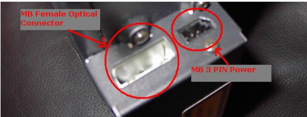
Back of CD Changer MC3010 showing the MB Female Optical Connector and the 3PIN power supply:
