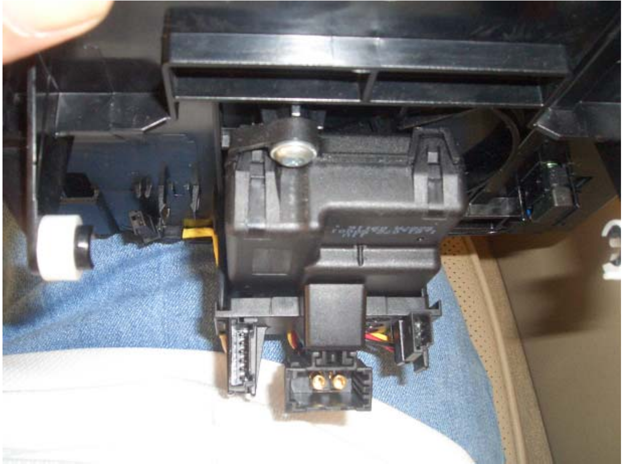
The following photograph shows the fiber optic connector and where the tab is.
