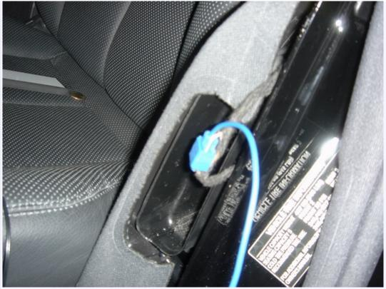
You want to connect the black wire from the EL transformer to the brown wire with white strip. Since the black wire on the EL transformer is not long enough, you need to get a piece of wire that is about 3 feet long (mine is the blue wire in the picture). Then you can use a tap splice to connect the extension wire to the brown wire with white strip.
