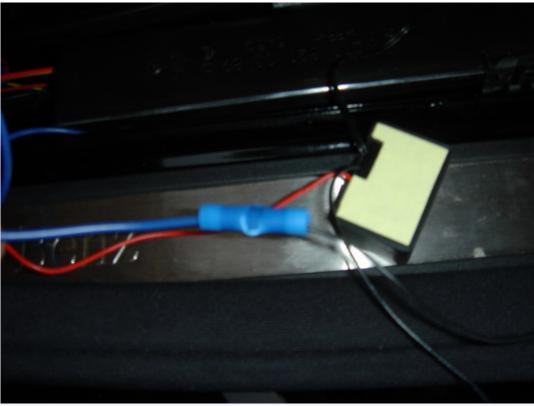
And then, just use a butt splice connector to connect the extension wire to the black wire on the transformer.
