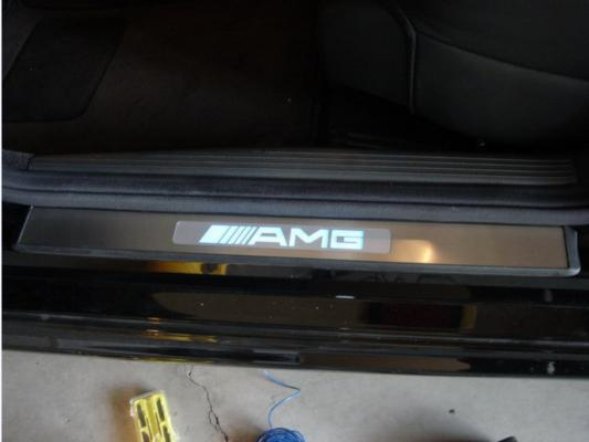
Remove the white protective films on the top of the illuminated door sill to reveal the brushed steel trim. Installation for the driver side is now complete.
