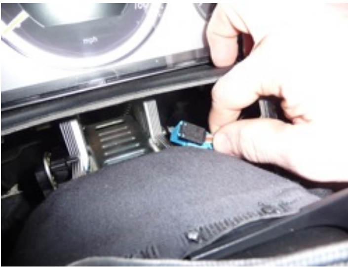
Locking clip secured
