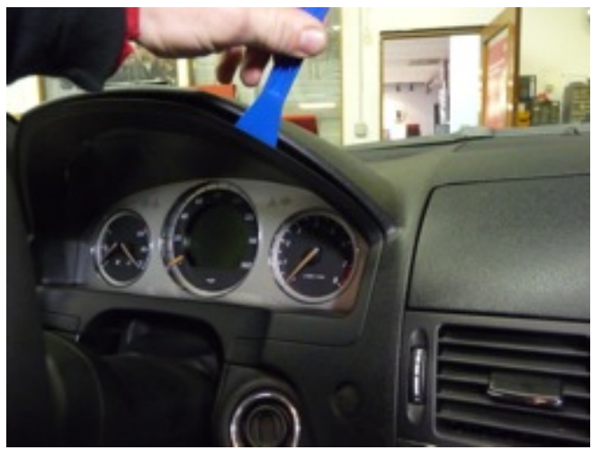
Unclip top right of cluster bezel
