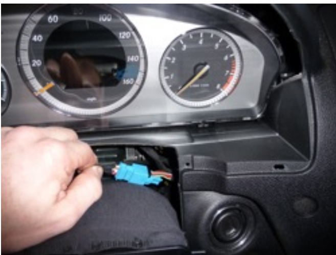
Plug harness in and into EIS
