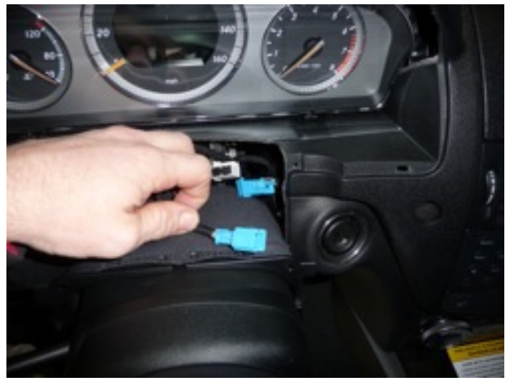
Route harness up to EIS from bottom
