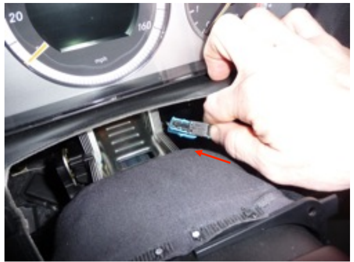
Slide locking clip in direction of arrow
