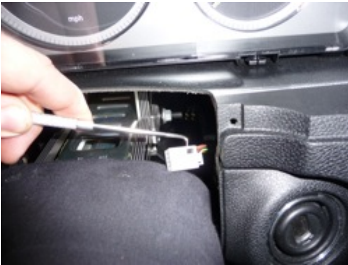
Remove white shroud from plug
