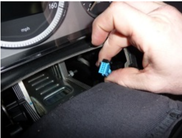
Install blue cover on OEM plug
