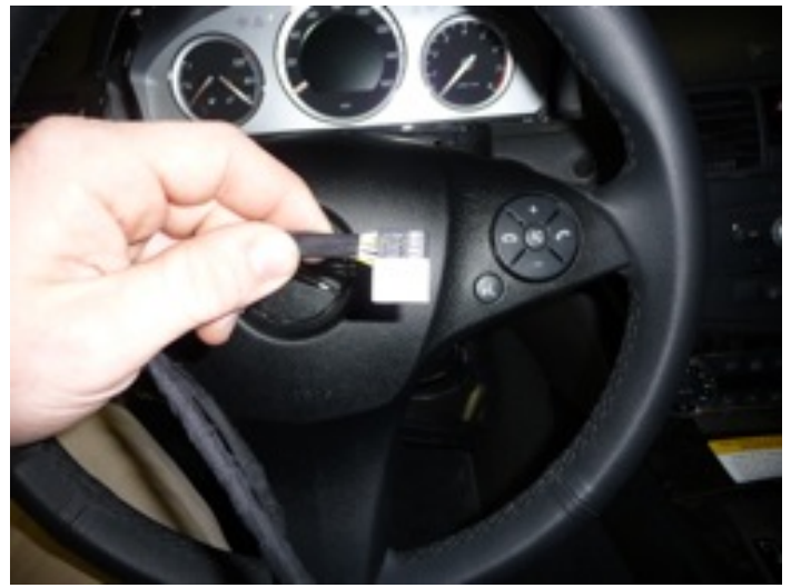
Install shroud on Smartkey Starter™ harness
