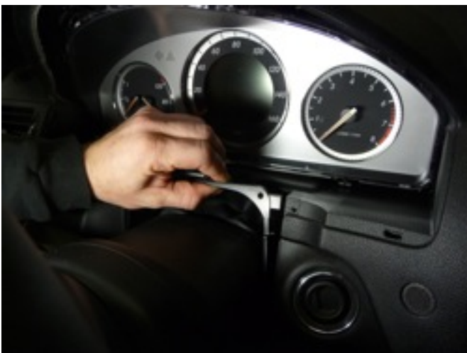
Unclip steering column boot
