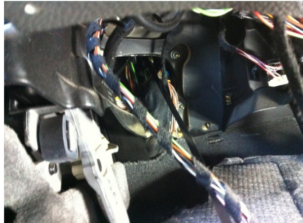
Wire Route (Driver foot well side)
