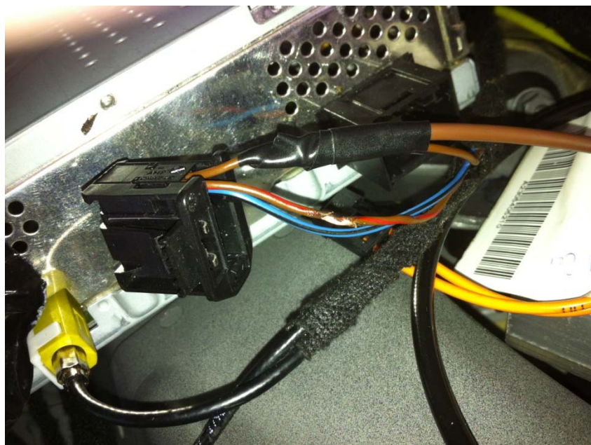
Tapping on Pins 2&4 on the Audio Gateway Fibre, Power and CAN connector
