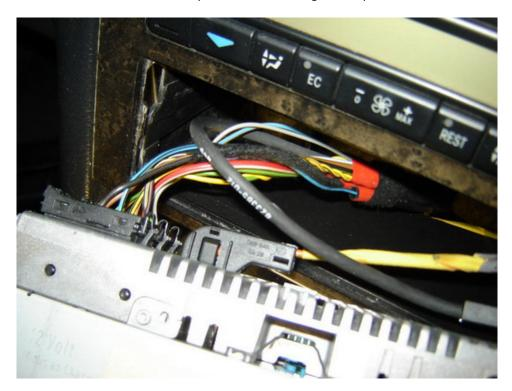
Follow installation instructions. Three connections required: standby/wakeup, power, ground. I shaved the insulation back on the factory harness, then braided in and soldered the Gateway wires after cutting them to length. Apply insulating tape. Insert the appropriate fiber optic loop into the system. The supplied loops are labeled for Command and non-Command systems so it is easy to know which to use.
