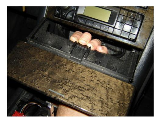
Next, use the radio removal tools to release the catches and carefully pull the radio out of the dash. Be careful of the fiber optic lines.
