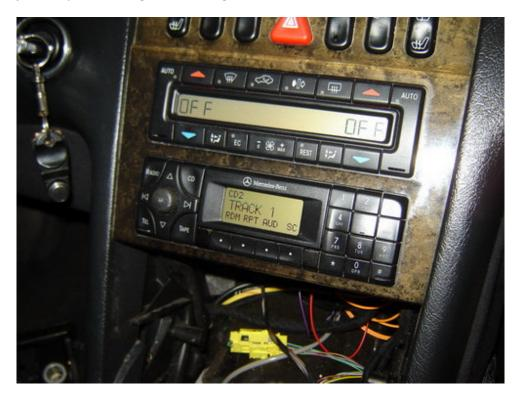
Reassembly is reverse of disassembly. One tricky point for me was getting the lighter connector back onto the ashtray; the harness was a bit short and it took me several minutes to fit it into place.
