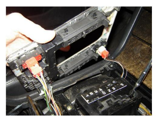
Remove two screws from ashtray, lift out and disconnect the lighter power connection. You will need to move the shift lever to the rear to have room to remove the ashtray.
