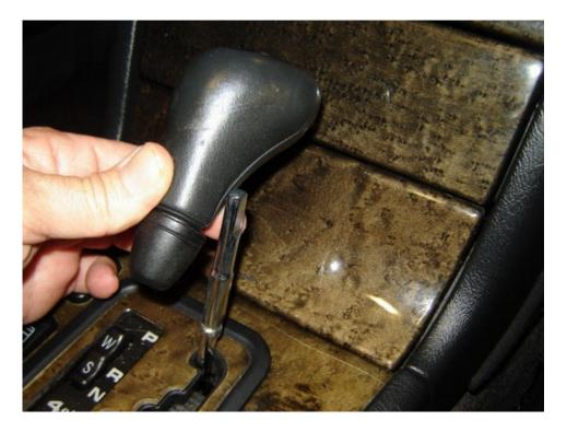
Next, pry up and remove the trim around the shift lever.
