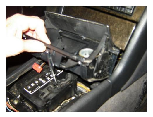
Remove center storage compartment. You will have to reach behind and above it to use your finger(s) to pull down on the center catch on top of the compartment.
