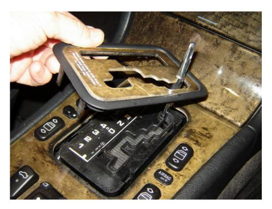
Lift large trim panel from the rear, then disconnect the electrical connections.
