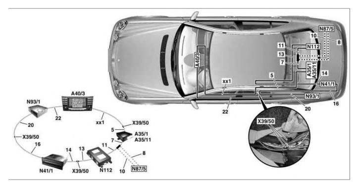
Shown is the routing of the fiber optical cables for Media Oriented System Transport (MOST) - vehicles as of 09/03 with COMAND, with SDARS (Dealer Option Kit) and without code 819, CD changer (6-disc)
