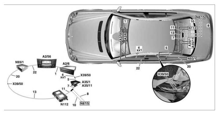
Shown is the routing of the fiber optic cables for Media Oriented System Transport (MOST) - vehicles up to 09/03 with Audio 50,
