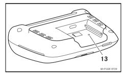
Using a pointed object, press in indentation (13).
