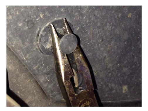
5) Once all 3 plugs are removed, carefully pry back the plastic cover. Note the green and brown wires, they are connected to the light bulb housing you will need unscrew in the next step
