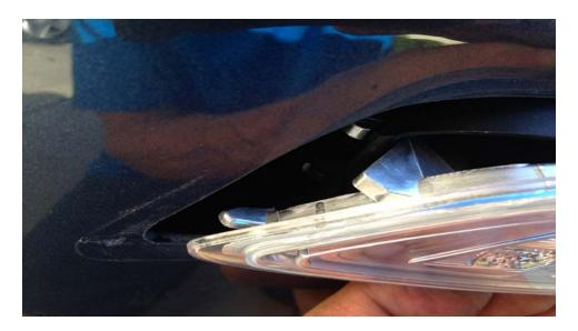
14) Once the 2 feet are hooked and the front clip has been slid securely to the <u>front</u>, then the rear-retaining clip is ready to be pressed until it "clicks". I recommend pressing gently on the outside of the housing while holding the inside body with your other hand. Don't press too hard – it should clip together easily. Once it is clipped, you're almost done. Now, we need to connect the LEDs
