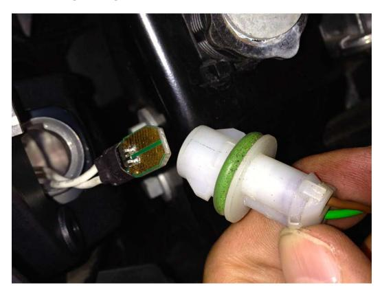
16) Now, you need to reinstall the bulb housing into the LED housing. Notice the 2 tabs on the white plastic housing? These need to be vertical when inserting back into the LED housing. Be gentle and once inserted all the way, a quarter turn (90 degrees) to the right should lock it in place.
