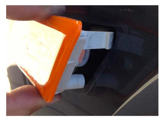
11) Now wiggle and pull the housing toward the  $\underline{rear}$  of the car in order to release the  $\underline{front}$  tab
