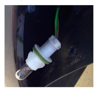
7) Pull the bulb out and discard or keep for another project. Note the blade fitting – no need to unscrew the bulb.
