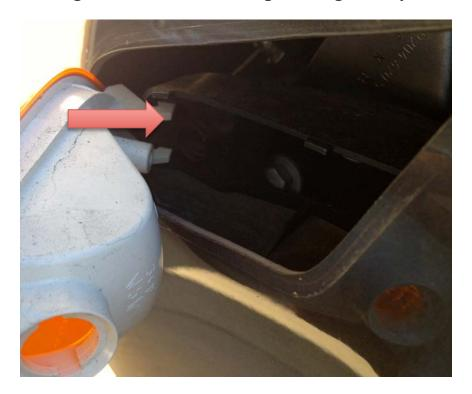
13) This step is the trickiest. You need to insert and hold the new plastic body inside of the fender. First, hook the 2 front feet of the housing as seen above, then make sure to fish the new wiring through the round hole in the plastic backing. Reattach the front of the housing to the fender (carefully!) by the front tab as seen below.
