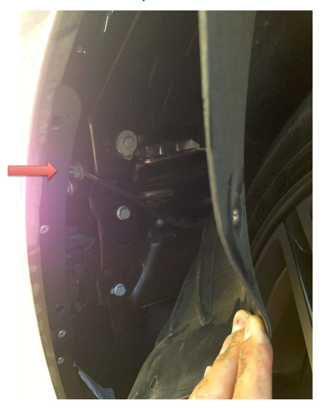
6) Reach in and grab the light bulb housing with one hand and gently twist 90 degrees until it unlatches. Try twisting to the left first. It should turn easily. Once out, it will look like this.
