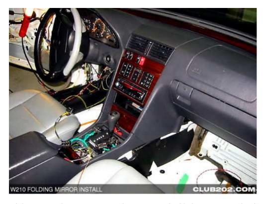
While running the wires its a good time to run the blinking wires up the doors to save time. On the MY 1995 we used for installation we've tapped the Black/White and Black/Green wires for the blinking portion. If you are unsure as to which wires colour your car uses for the blinking to the rear lights use a multimeter to figure out which wires you will need to use.
