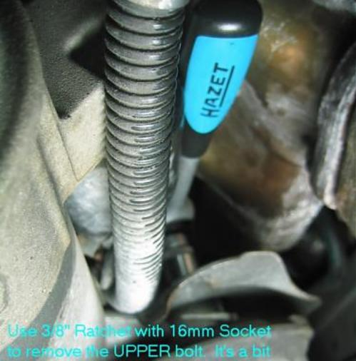
Use 3/8" Raigher with 16mm Socket to remove the UPPER bolt. It's a bit of a work space. IF you can get your bands on a 72 tooth (FINE) ratchet, the better!
