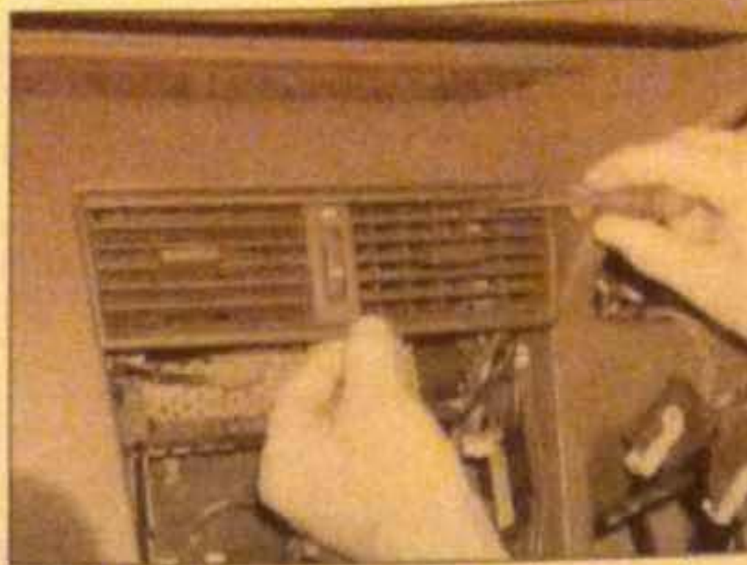
10.8b ... then prise down the upper clips and remove the centre vent assembly
