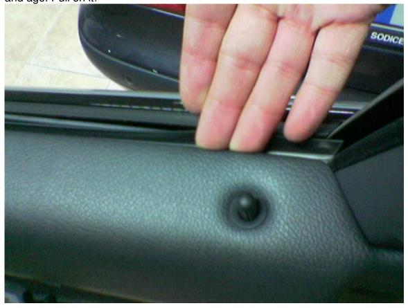
7-remove the cable from the pull handler- Note open end on white plastic piece- must go back same way or the door handle will protrude slightly- An extra hand at this point is helpful
