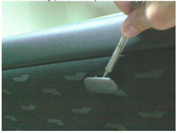
2-Under the door arm rest there is a cover, pop it off and remove the screw- T30 (drop the window)
