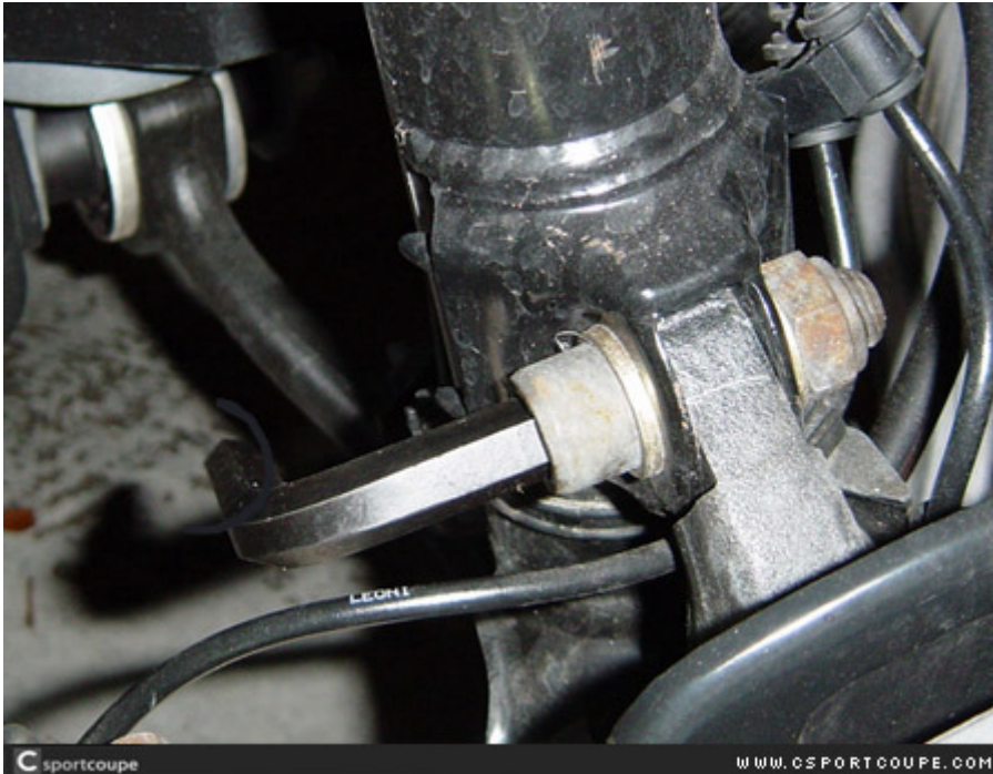
Remove middle clamp using a 12mm hex wrench.
