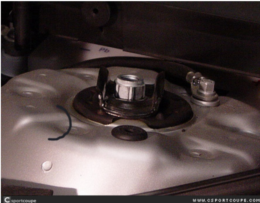
Remove the Top strut nut with a 22mm socket. Edit: Something about this was wrong....
