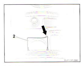
2. Carefully lever out the drinks holder (2) with a screwdriver (see arrow) and remove.
