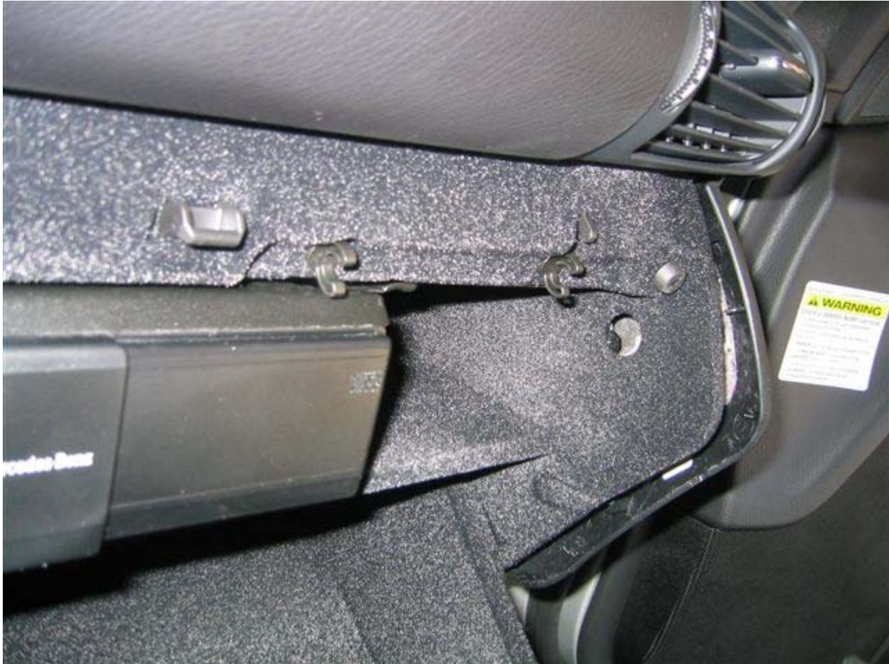
4. The hole is for fitting the AUX-plug of the cable harness.
