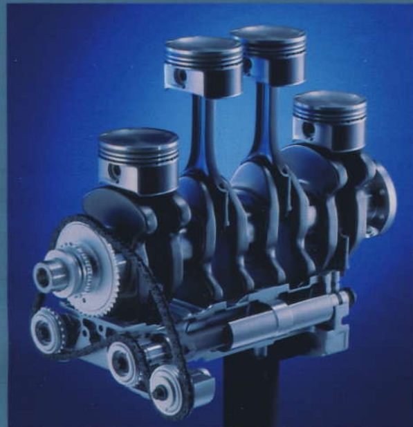
Above, left: two shafts, carrying suitable protrusions, rotate at twice engine speed parallel to the crankshaft, to balance the secondary vibrations in this four-cylinder diesel. Below, left: the percentage of sound absorbed by the various components of the interior trim is shown here graphically. Above: the sketch illustrates wave terminology.
