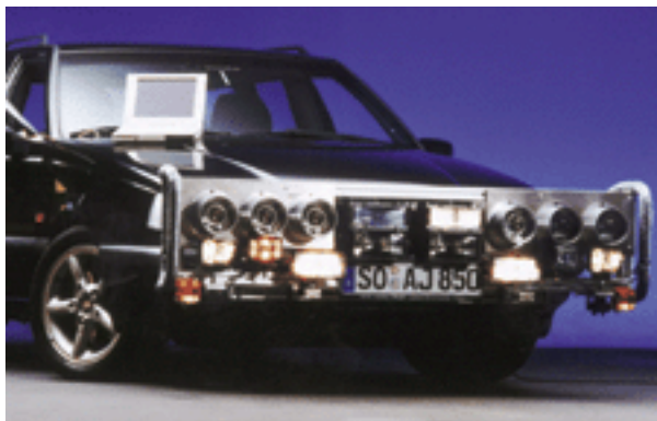
Carrier bars hold a range of lamps for studying adaptive front lighting systems. Early into the Eureka study, test bars helped researchers answer initial questions.
