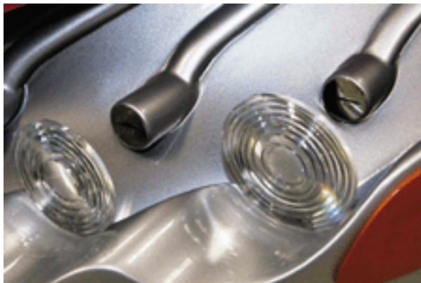
Lights out in front: Hella developed prototype headlamps for the Volvo SCC, Safety Concept Car. Glass fiber bundles guide light from a central xenon source out to three Fresnel lenses.
