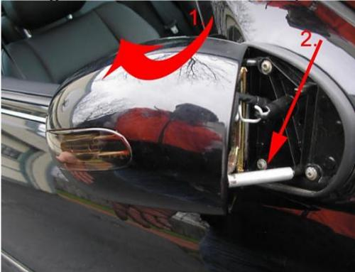
4. insert a long flat blade screw driver from the front end of teh vehicle into the mirror housing. locate a molded in key way to a small .75 inch vertical metal tab. move that tab inboard toward the vehicle and gently begin to slide mirror housing back. to not bend the spring clip - that is the retainer for the mirror housing unit.
