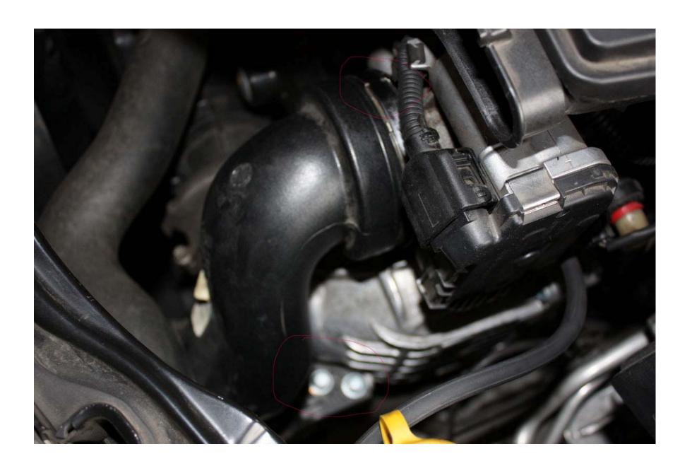
The hose clamp is easily removed by using a flat headed screwdriver.
