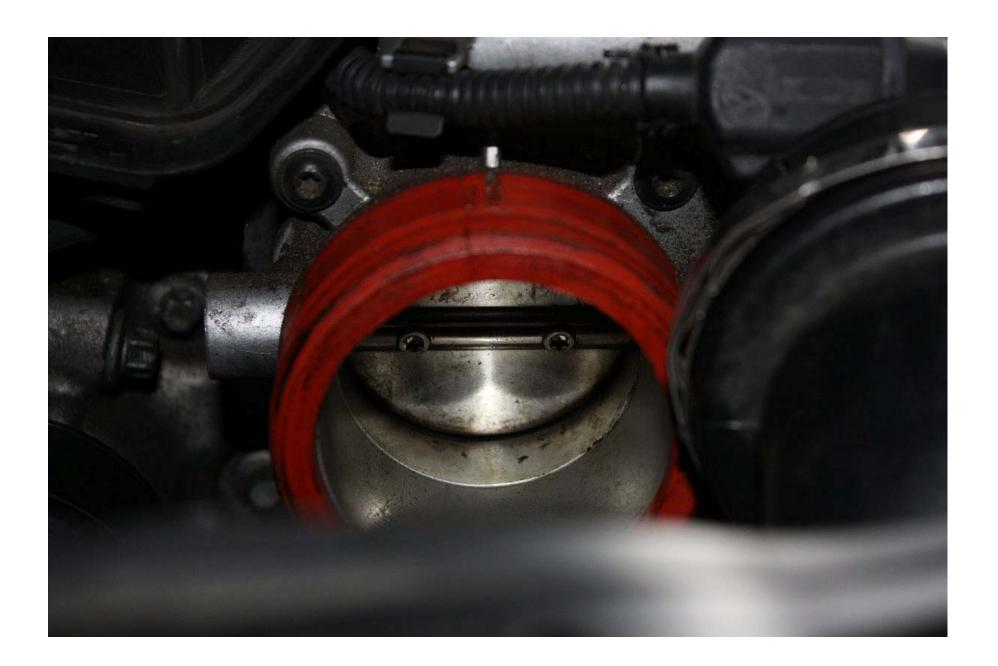
We cleaned it off with paper towels and q-tips and a couple light sprays of throttle body/air intake cleaner:
