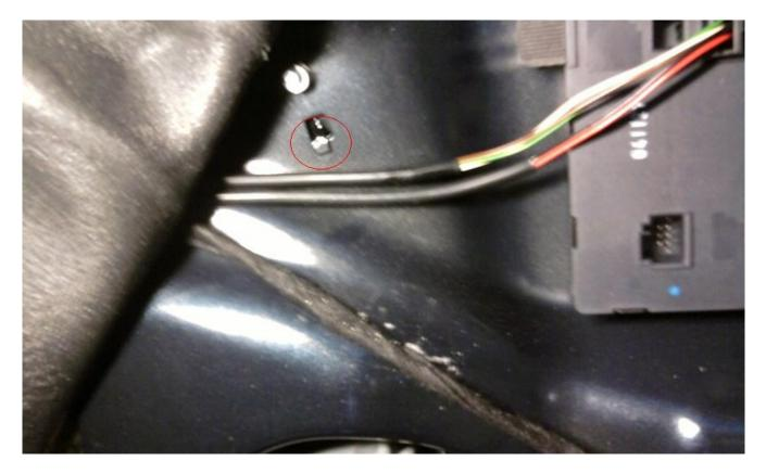
Near the top of the door, the top cable will need to go inside this holding bracket so it doesnt rub w/ the window(see pic).
