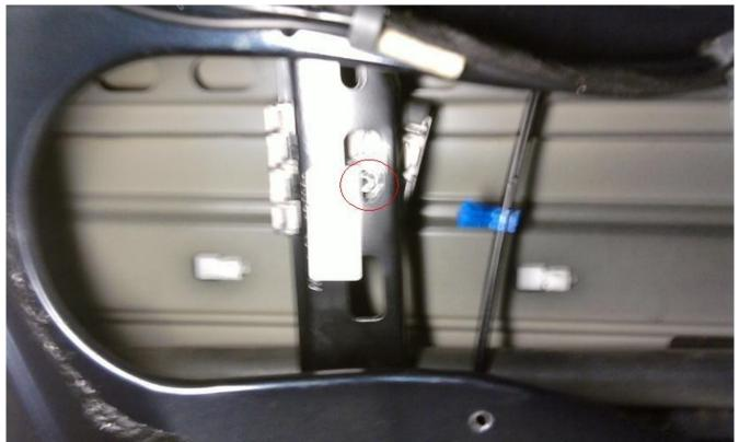
(notice the blue clip, clip this into the  $2^{nd}$  opening after you've installed the regulator)
