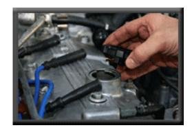
Step 2 - Figure out which spark plug adapter works best and connect the gauge into the hole. Put the vehicle in gear and set the parking brake to prevent the engine from turning when air is compressed into the cylinder. Start with the regulator turned counter-clockwise to zero the incoming pressure. Connect compressed air. Turn the regulator clockwise to pressurize air into the cylinder.
