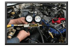
Step 3 - Record leakage percentage for the cylinder. Remove the oil dipstick, radiator cap, and oil filler cap. Open the throttle body or remove the air cleaner. Listen and watch. Wherever air is escaping will indicate where the problem is. Disconnect the gauge and move onto the next cylinder.
