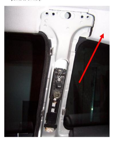
4. The C Pillar pulls off similarly to the B pillar. Start with the front and then slowly pull off as you move to the rear. Once you pull the clips out, pull it forward towards the front of the car to pull it up and down. It will hang down since the rear seat belt is still attached. Here's what you'll see (the amplifier is circled, arrow points to the some of the plastic clips that hold the C Pillar on):
