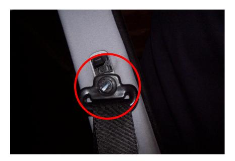
2. Remove the bolt with a 17mm socket. Once you remove the bolt, then you can pull off the B Pillar. Just gently pull and it will come off and then it lifts up and out. Here is a pic of it partially pulled off:
