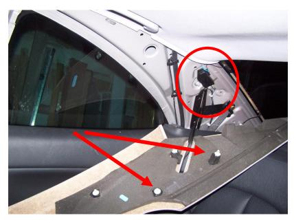
5. Here is a close-up of the antenna amplifier. There are 3 connectors and one bolt. The black clip on the top is removed by pinching the clips, the plastic clip on the back just pulls off, and the other connector screws off. Once you've disconnected the 3 clips, then remove the bolt (10mm).
