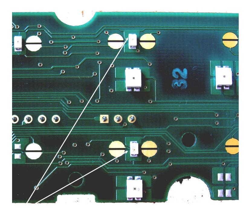
Notice the orientation of the LEDs for polarity. The dark "dot" goes towards the outside edge of the PCB.
