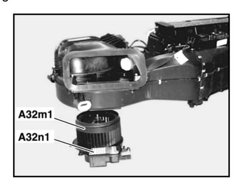
NOTE: Blower motor is switched off while cranking engine.
