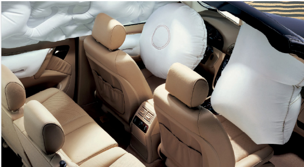
Demonstration of available airbags in the M-Class (W 163). The accident-specific circumstances determine which airbag(s), if any, will deploy.
