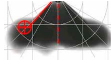
Figure 4: Spray Formation Recirculation Zone
