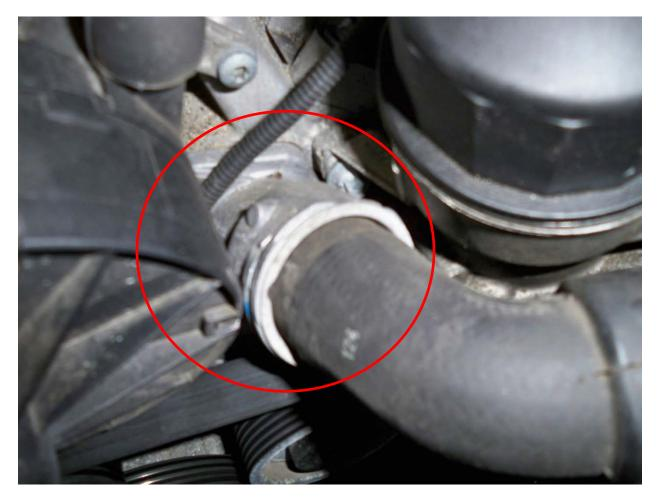
To remove the hose just slide the clip out on the hose connecter. No need to remove the clip. The clip holds the hose on to the thermostat. Once the clip is released, you can pull the hose out from the thermostat body. May need some force to remove. See picture below.
