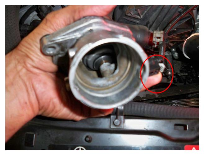
Here is the failed thermostat. Notice it stays open. It should be closed and only open when the temperature reaches above 85°C.
