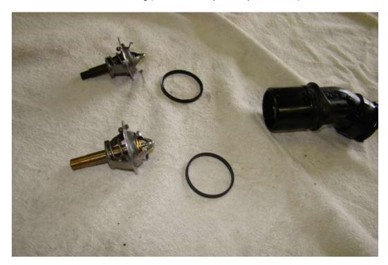
Place the new O-ring on the t-stat housing.
