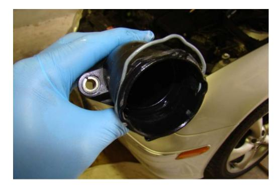
Insert the T-Stat housing back on the engine block and re-screw the bolts.
