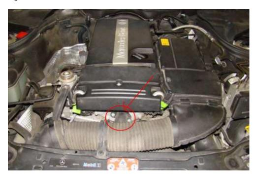
Pop each side by placing you hand underneath it and pull towards you. This should easily come out.
