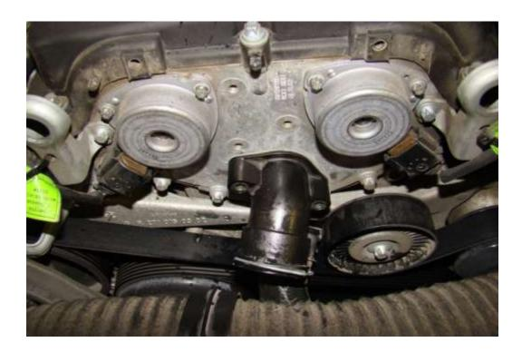
Also remember to reconnect the radiator hose and press down on the medal clamp, as shown below:
