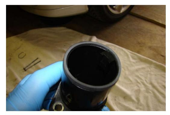
When placing the new T-stat, be careful as it only goes in one way. There are a couple of tabs inside the housing. \* DON'T FORCE IT IN! \* Again, it only goes in one way.
