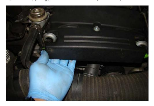
Now using a small flathead screw driver remove the hose clamp. If you accidentally remove the metal clamp, don't worry, you can place it back later.
