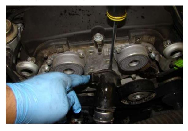
The pictures below show the T-stat housing with the old T-Stat in place and the engine block and connecting hose.
