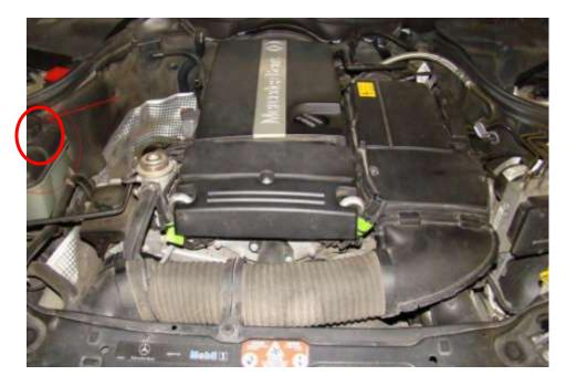
Next; at the front, right side, underneath the engine you will find a RED plastic bolt and black plate. Affix your plastic /rubber hose to a nipple behind the black plate. See arrow below.
