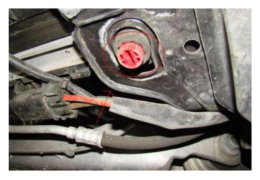
The picture below shows the placed hose. Now use a flathead screwdriver to turn the red plastic bolt and release the coolant. Be gentle with this red bolt! (Brake it and you'll have coolant everywhere!)
