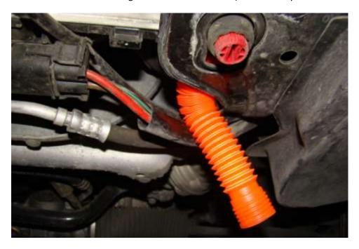
Notice the coolant flow (total should be about 1+ gallon). Also, keep the tray nearby. When you remove the Thermostat housing (later) more coolant will come out! (Some splashed next to the tray).
