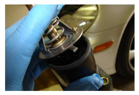
Remember to place back the hose clamp we removed in the beginning. Don't force it close. Leave it like the photo. You will force it close once you have inserted the radiator hose from where you removed it earlier.
