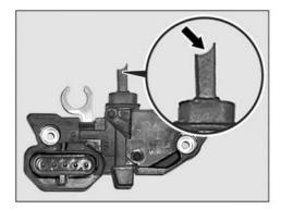
Inspect wear shape (arrow, Figure 18) of carbon brushes: If brushes have worn at an angle (arrow), alternator bearing damage is indicated and the alternator must be replaced. If brushes wear is normal, continue with regulator replacement.
