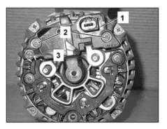
Remove three Philips head screws (2, 3, Figure 17); remove voltage regulator (1) from the alternator.
