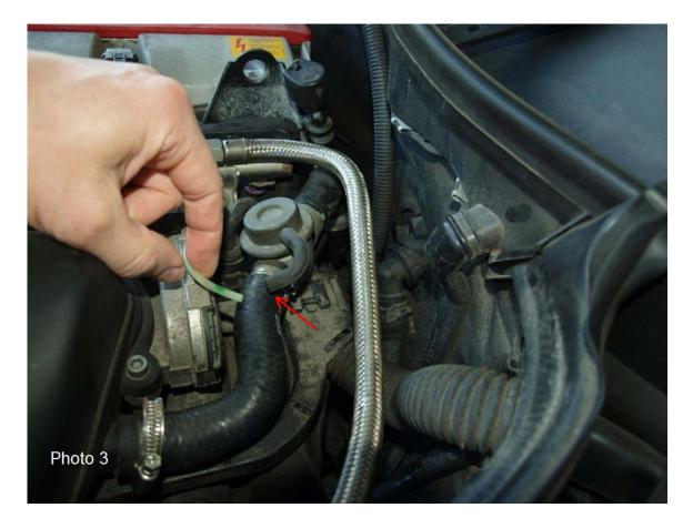
We need to check if there is vacuum suction on the output of the vacuum valve, i.e. finger should stick.
