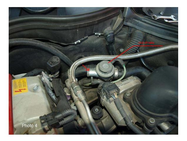
The next and last unit in the chain will be a check valve (see the look on Photo5). This valve, let's say, has one-way air conduction. It allows air to flow in the direction from the compressor to exhaust manifold, and not in the opposite direction.
