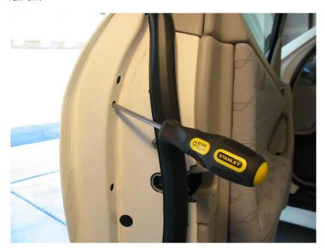
Step 2: Use masking tape to hold the screwdriver in place, so that you can continue the process without worrying the screw falling off.
