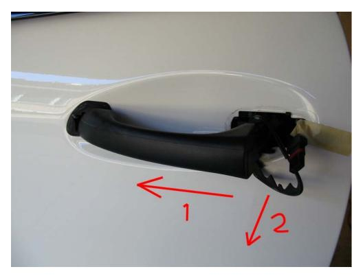
Step 5: Slightly pry the 3 hooks of the cap to remove the the lock and IR sensor.
