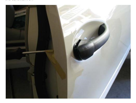
Step 8: There is no lock on the passanger side. Use a flat head screwdriver to pry off the spring holding the IR sensor to the cap.
