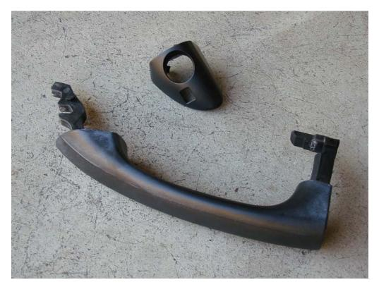
Step 7: (Passanger side) Repeat the procedures to remove the IR sensor assembly and the **handle** piece. Remember to tape the tail of the fastening screw first before removing the screwdriver!
