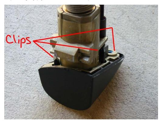
Step 6: IR sensor/lock cap removed.
