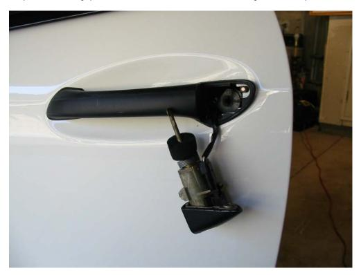
Step 4: Hold the screwdriver, and tape the tail of the screw to secure it. Now you can remove the screwdriver. Then slide the **door handle** out in the order shown.
