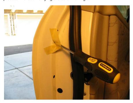
Step 3: Carefully pull out the IR sensor/lock assembly and unclip the sensor.
