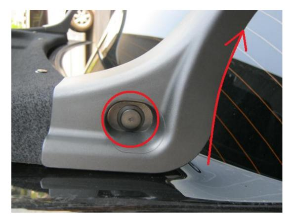
Also remove clips on each side of the arm cover and slide it down.
