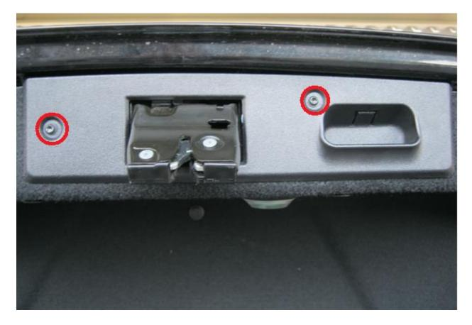
Pop the trunk and remove these two screws with T-20 screwdriver.
