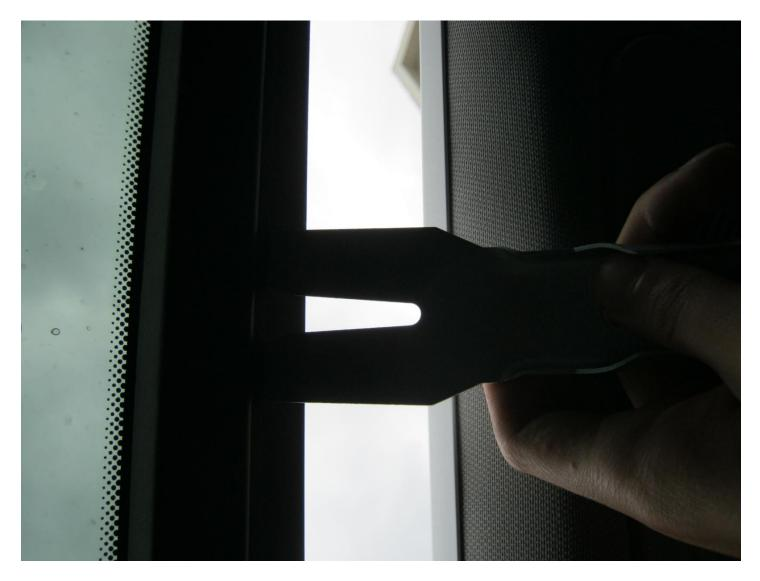
Open the roof about 10" and use plastic wedge (or something wide and thin) to pry out the front cover, start from the center and work it out to each side. Do not use screwdriver because you'll put too much stress on one spot and break the cover.
