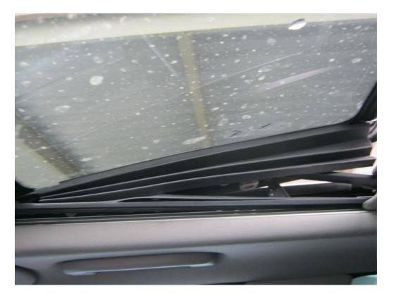
Now, put the roof in tilt position and pull the torn side cover off. Make sure you memorize the position before you pull it out.
