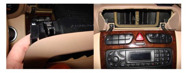
11. Again, grab the flashlight and now look under the remaining section of the wood trim around the Radio/Command. You should be able to see a small metal loop on either side. Use one of the screwdrivers to pop each one down but not completely out. Doing this, should release the remaining section of the wood trim around the radio. Unplug each connector, but again, mark or remember where each connector came from. There should be atleast 3 connectors depending on your options.
