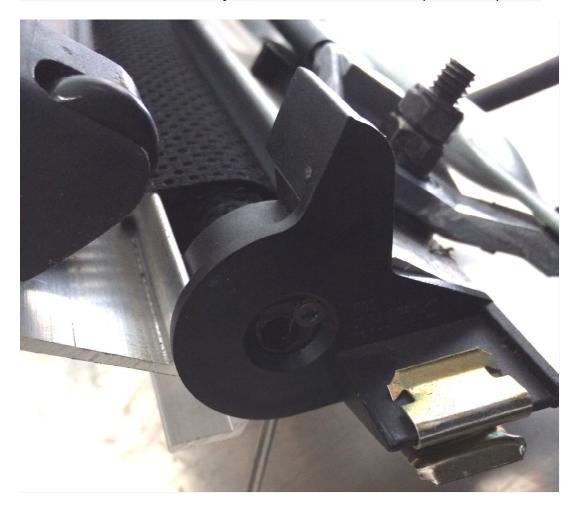
3) drill out the rivet with the 5/32" drill bit. Be careful to drill the center of the rivet, not make an oval hole.
