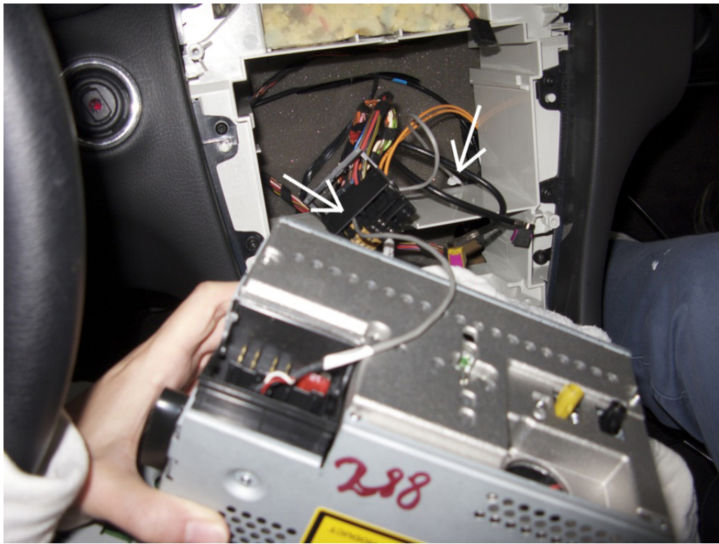
Figure 10: Wire Route Path in Center Console
