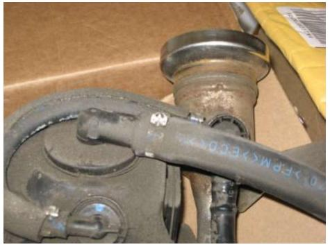
The original part uses black plastic where the foam-covered hose mates to the body of the filler assembly. Maybe the white plastic is more flexible and less susceptible to cracking.
