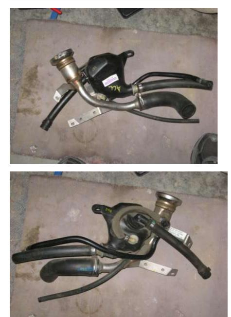
Updated part – note the white plastic connecting the foam-covered hose in the center to the body of the filler assembly.
