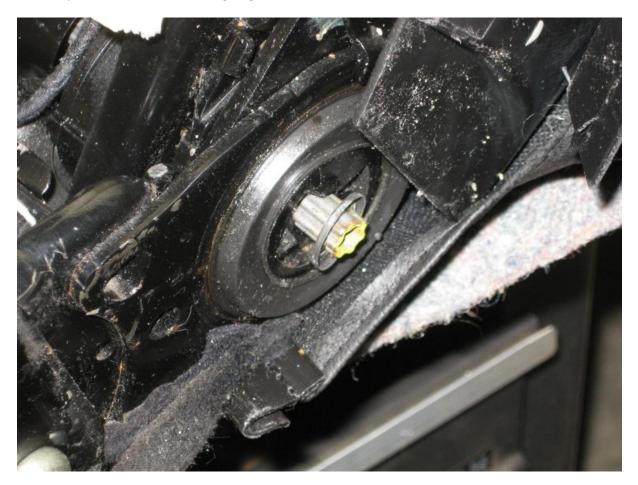
The problem I had was aligning the rod and the motor so that the rod would go into the replacement motor. I ended up powering the seat using a computer power supply and "bumping" the control until the motor aligned with the rod. It was a "fiddly" job. I recommend that you avoid it if you can.
