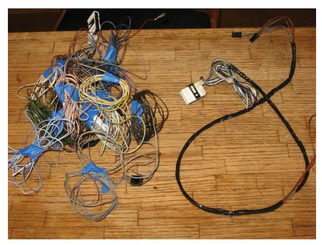
The big white and black connector that you can see in the middle of the picture fits into the memory module under the seat. The two smaller black connectors at the top right of the picture fit into the control unit in the door sill. At the extreme right of the picture, you can see a brown wire and a red wire with a black stripe. These provide the power and ground for the illumination of the buttons in the door sill control unit.
