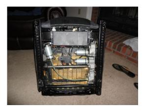
Here's a close up of the control module under the seat.
