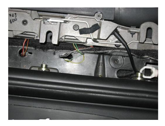
Push the connectors into the corresponding spots in the control unit and then reinstall the control unit in the door sill. Reinstall the seat and check for proper operation.
