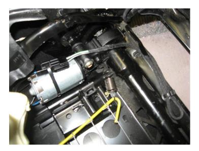
You need to peel back the upholstery from the bottom of the seat back in order to find it. It is attached to a rod that controls the seat function. You need to remove the torx fastener that holds the motor in place and then remove the retaining ring that holds the rod in place in order to remove the motor. Here's a picture of the rod retaining ring:
