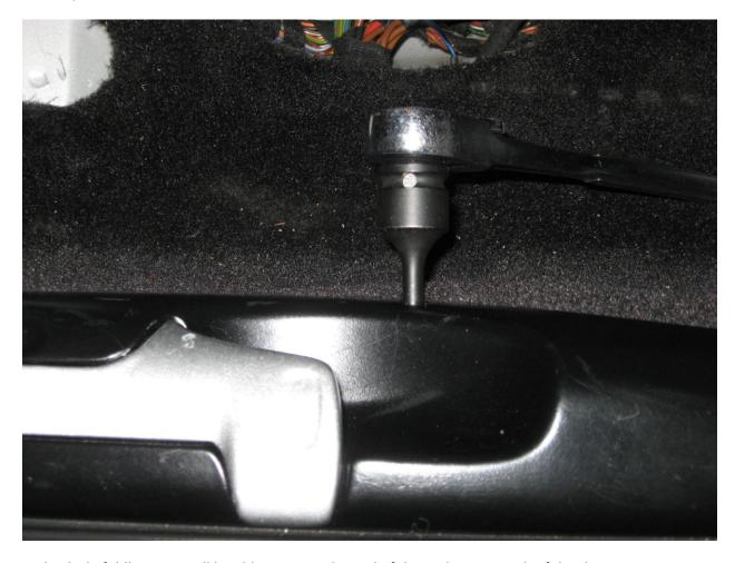
With a little fiddling, you will be able to insert the end of the socket into each of the three retaining bolts. Loosen, but don't remove them. When they are loose, you can pull the control unit out of the door sill.
