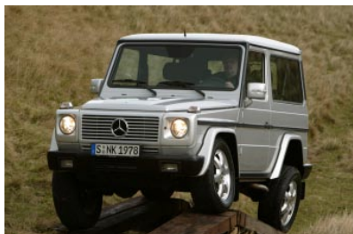
The G-Class is a classical off-roader and is the only vehicle to provide three locks
