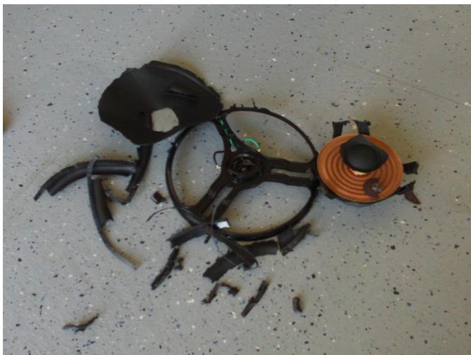
Using the Dremel took cut through and remove the inner 3 leg supports as close to the inner aluminum door panel as possible. This is not difficult to do the grinding wheel cuts like a hot knife through butter.
