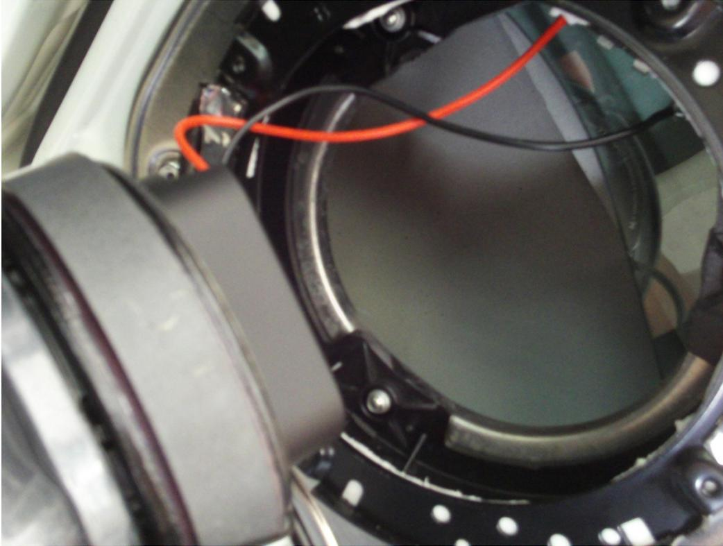
Install the speaker with the 4 fine machined screws into the assembly ring.
