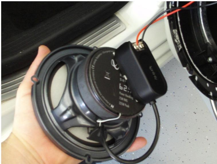
Attach the cross over unit to the bottom of the speaker magnet to clear the window glass after installation.
