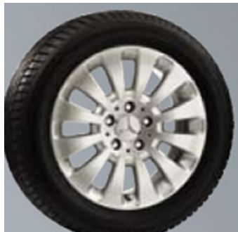
12-spoke wheel | 16 (A204 401 0602) > Titanium silver - Wheel: 7J x 16ET 43 Tyre: 205/55 R16
