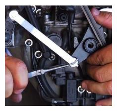
Install left & right side metal lever. Do not use excessive force. If the ball does not snap in easy, center spring clip then apply pressure and ball will click in. Install center bolt (torque to 80in lbs./ 9nm) with Loctite on threads only. **NOTE:** Do not over tighten. This can crush shoulder on bolt and cause bending at lever.
