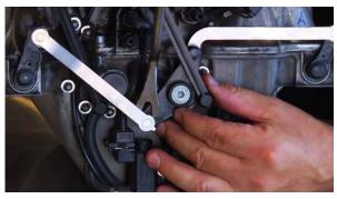
Carefully disconnect the left & right side metal lever. Remove broken ball from plastic actuator rod. Remove center bolt (torque #30).
