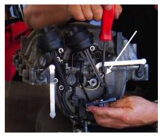
Check that lever moves freely and that lever does not interfere with stud. \*If stud does interfere with lever, trim stud slightly until it clears. DO NOT REMOVE the stud all the way since it retains the wires.\* Install actuator plastic rod on ball. Replace intake manifold gaskets. Install manifold according to Mercedes Benz procedure and torque valves. Clear codes in system.
