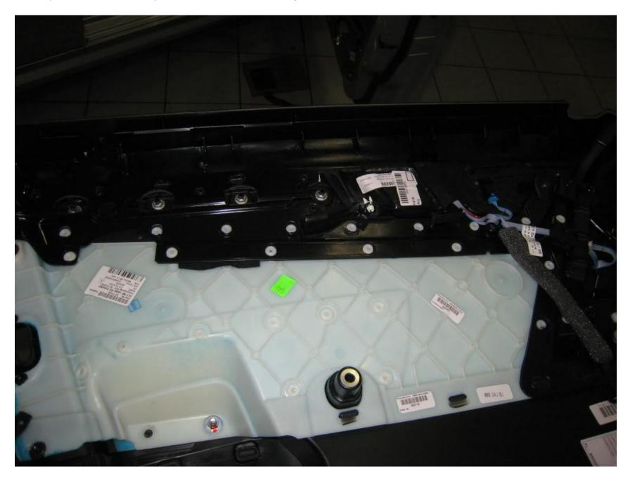
For the seat control trim piece, remove the rubber sticker overlying it's white harness and undo both the white and blue harness. The trim piece along w/ the seat control mechanism (w/c is the back and butt control connected by some silver wire) can now be freed up from the door panel by undoing the trimpiece's tabs from the back of the panel -- a plastic frame will be left behind on the panel as shown below.
