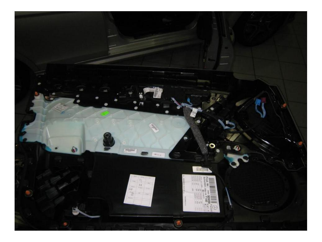
The top of the door panel is rubbery and is kind of hinged onto the metal part of the door; you just pry it up and out. As you remove the entire door panel, the lock post comes out from under it's hole.
