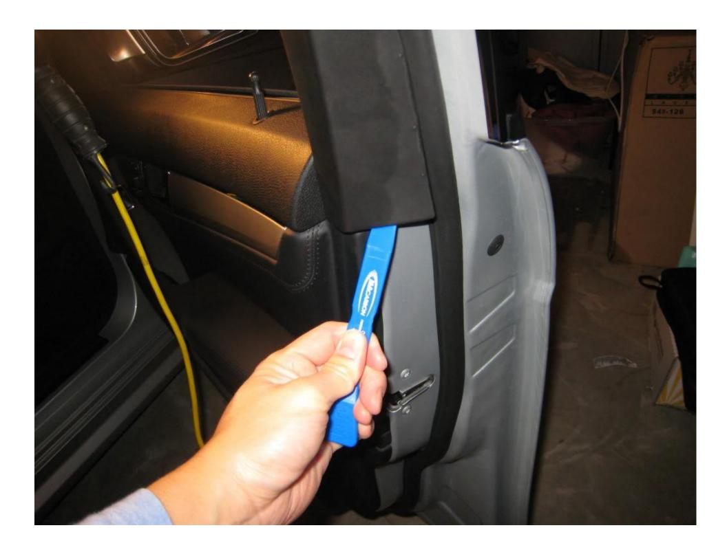
This will reveal this funky rivet (PN: A0009917940). It is square, with an inner pin and an outside lock. Pry out the inner pin turn it 90 degrees and reinsert it into the outer lock part (there's a center stripe across the front of both parts that guides you somewhat. This unlocks the outer part and you can then remove the whole rivet. NOTE: I did not find that one is able to reuse this rivet once it's removed ie I wasn't able to pull out the inner pin out after doing the above procedure.
