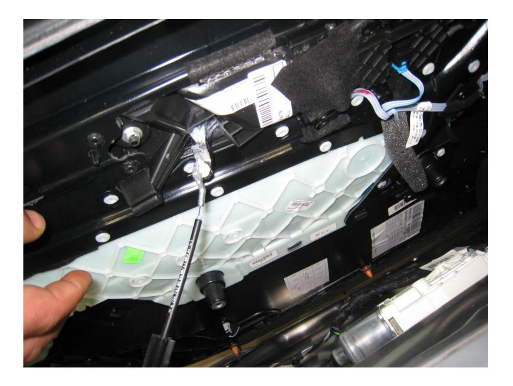
The door panel is now free; lay it upside down on a soft surface. Unscrew the 10mm hex bolts shown below for the long trim piece and seat control piece. The former will just come off after unscrewing.
