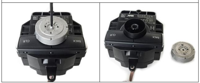
Step 5: Remove the knob screw with a T10 screwdriver.
