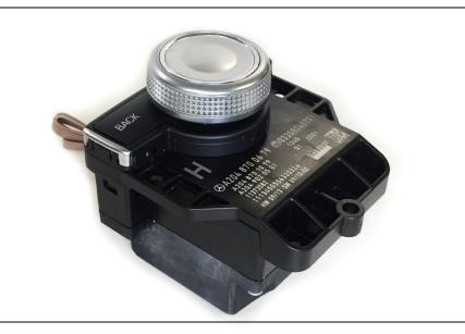
Step 2: Remove the knurled knob cover with a flat screwdriver.
