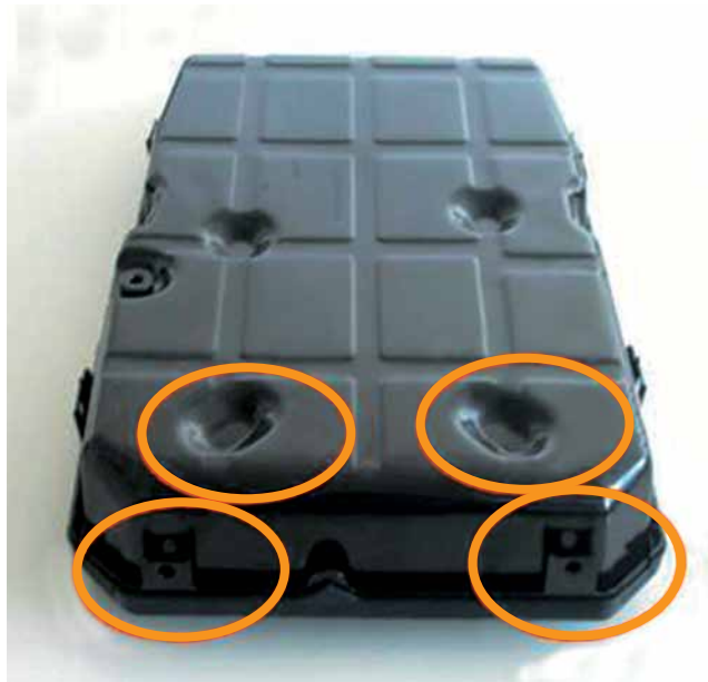
Oil pan 722.9 as of prod. 21.06.2010 Part no.: A222 270 05 12 Two oval and two round depressions in the oil pan and cable clamps
