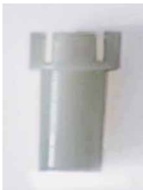
Overflow pipe in oil pan is white
