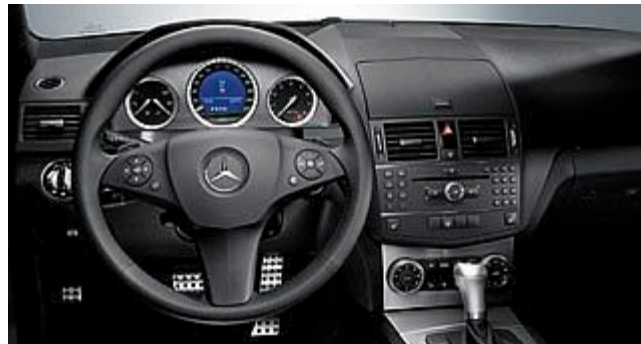
Behind the 3-spoke leather steering wheel are shift paddles for manual gear changes (in conjunction with automatic transmission)
