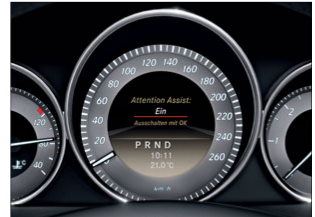
Helps to detect drowsiness at an earlier stage. ATTENTION ASSIST can remind the driver to take a break
