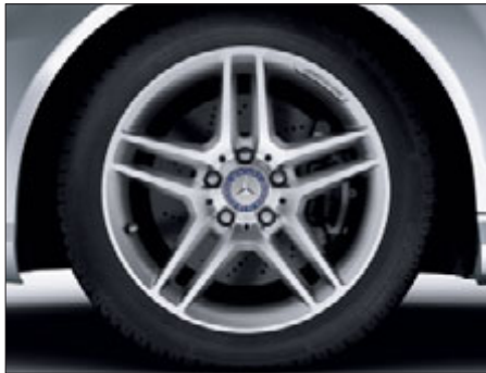
5-twin-spoke AMG light-alloy wheels with 225/45 R 17 front tyres and 245/40 R 17 rear tyres, with high-sheen finish (part of the optional AMG Sports package, not for C 63 AMG, Code 784)
