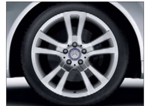
incenio 5-twin-spoke light-alloy wheels with 225/40 R 18 tyres at the front and 255/35 R 18 tyres at the rear (accessory)
