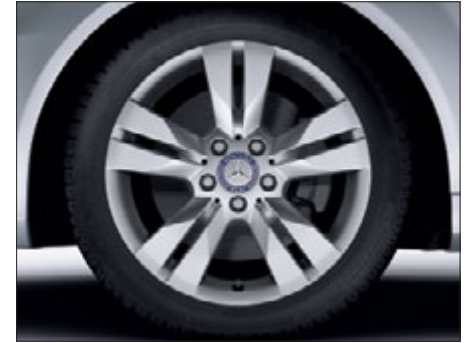
5-twin-spoke light-alloy wheels with 225/45 R 17 front tyres and 245/40 R 17 rear tyres (optional, Code R52)
