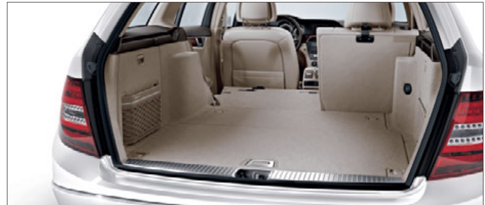
The rear bench seat can be split 2/3 with just one hand to give a versatile stowage space
