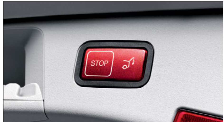
You can also open and close the EASY-PACK tailgate in a low position at the push of a button
