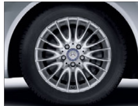
Multi-spoke light-alloy wheels with 225/50 R 16 tyres (optional for 4-cylinder models, Code 43R)
