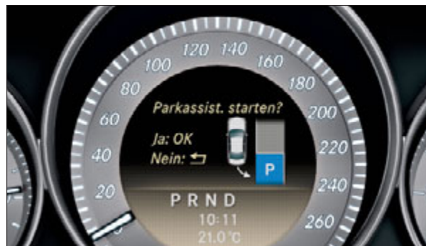
Parking Guidance automatically calculates the length of parking spaces at speeds up to 36 km/h
