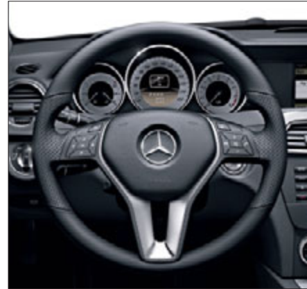
3-spoke multifunction steering wheel with 12 buttons in nappa leather, perforated in the grip area
