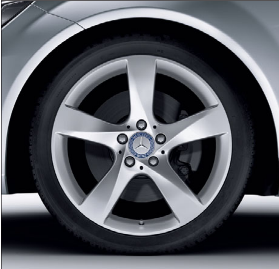
5-spoke light-alloy wheels in sterling silver with 225/40 R 18 front tyres and 255/35 R 18 rear tyres (optional, Code R36)
